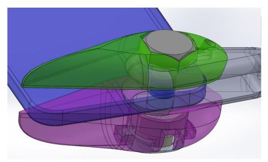
Step 2: Disassemble the installed rudder clevis bolted attachment.
