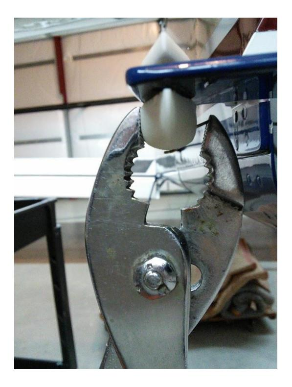
Step 8: Install small button on bottom fairing. Insert the button tang to aft side of the bottom fairing and snap into position.
