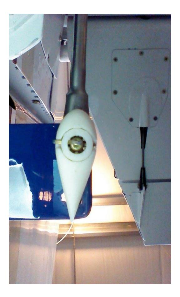
Step 9: Verify the rudder moves freely with no interference to the fairings.
